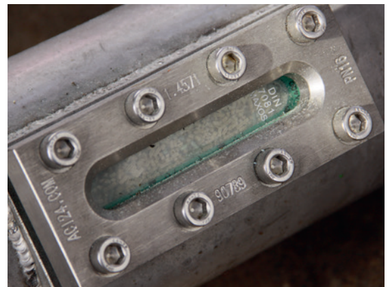
Continuous monitoring of the material flow from the Dense Phase Conveyor upwards to the specially designed filling hopper
